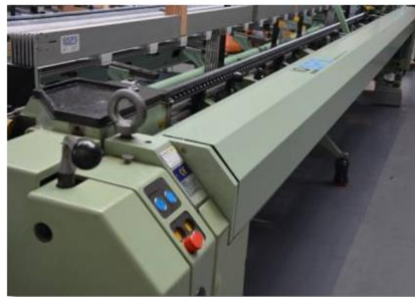
Pic: Special weaving machine, width 5.40m by IQ-SPS
